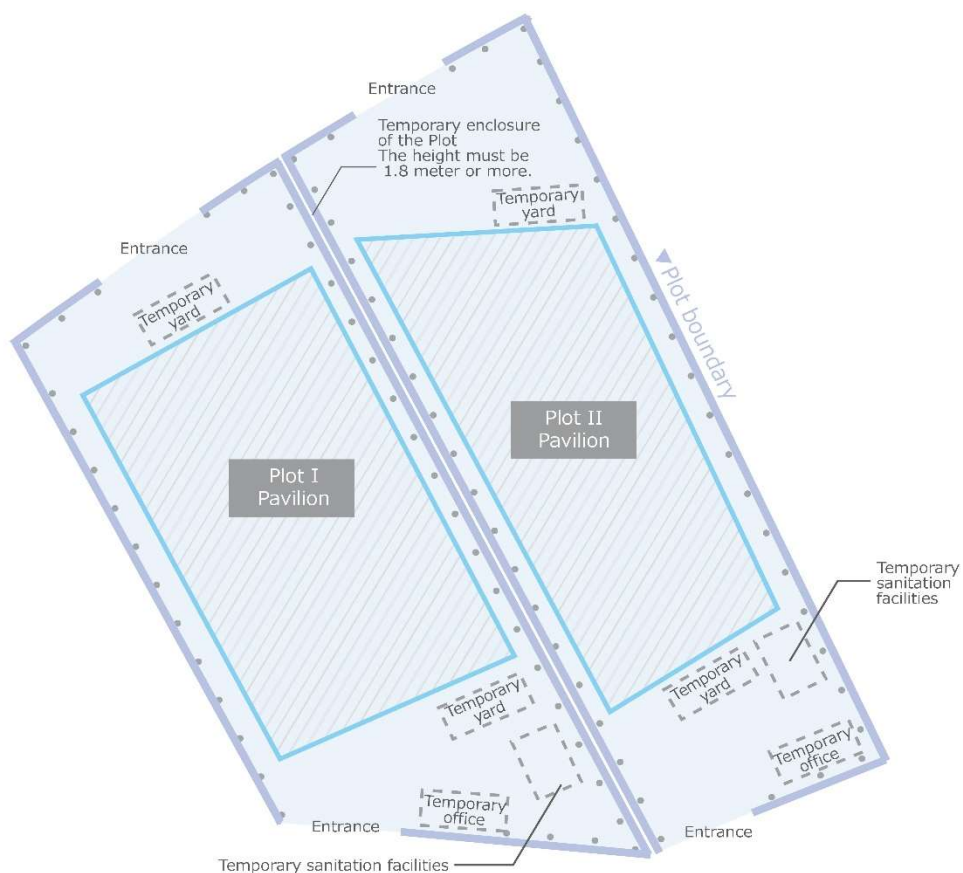
Figure 2.3 Overview of Installation Plan for Temporary Construction Facilities Within Plots such as Temporary Enclosure
